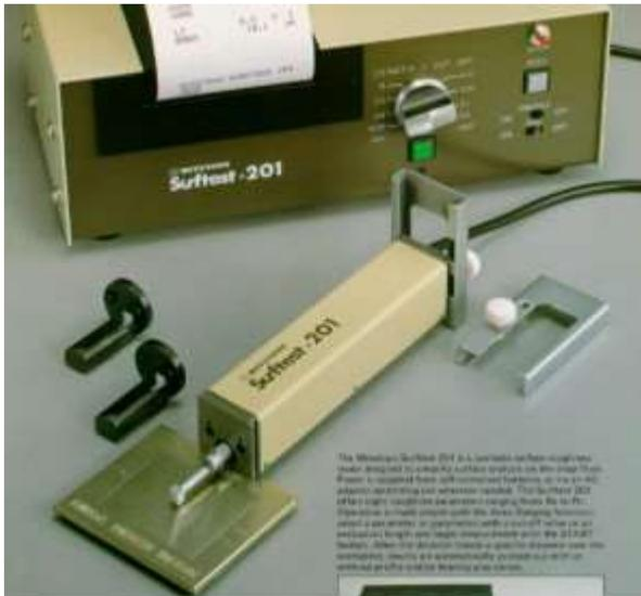
*A profilometer is an instrument that measures the actual metal surface by dragging a stylus across the metal a predetermined length, measuring the distance between the peaks and valleys of the surface.*
